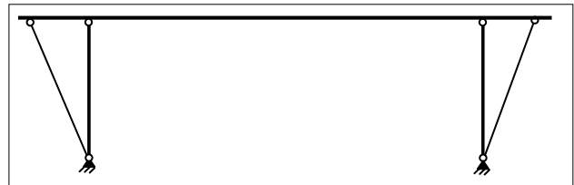
Figure 7: Indeterminate frame system with V-shaped frame corner
